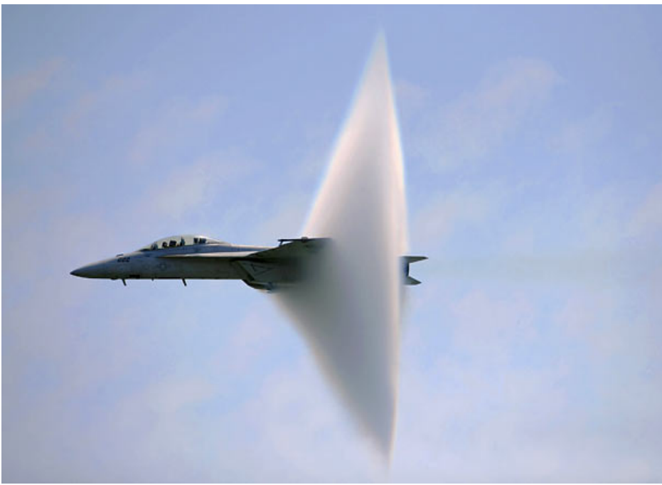
An F/A-18F Super Hornet hits the speed of sound. As the plane pushes air away, the temperature drops and water vapor in the air forms a ring cloud around it. – Time Magazine
